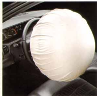
A standard driver air bag, in conjunction with three-point seatbelts, can help prevent injury in certain severe frontal impacts.
