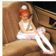
With the standard rear seatbelt child-comfort guides, you can adjust the shoulder belts to fit young rear-seat passengers and make safety more comfortable.
