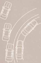
Standard anti-lock brakes help maintain steering control and prevent skidding when braking on most slippery surfaces.
