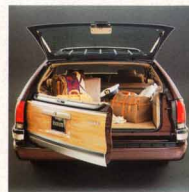
When using the rear seat, the tailgate opens like a car door for easy exit and entry.
