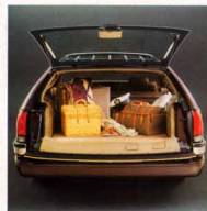
Roadmaster's tailgate opens down to enable easy loading of large and heavy objects.
