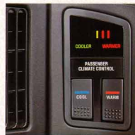
Dual automatic ComforTemp climate control enables both driver and passenger to vary their own individual temperature levels by as much as four degrees.
